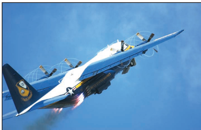
A JATO takeoff roll, showing rockets.
