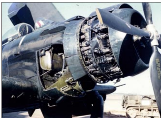
With part of the cowl removed, the powerful Wright R-3350-26 radial engine can be viewed. This was taken in late 1952 at K-6 airfield. (Credit: Richard Hawley).
