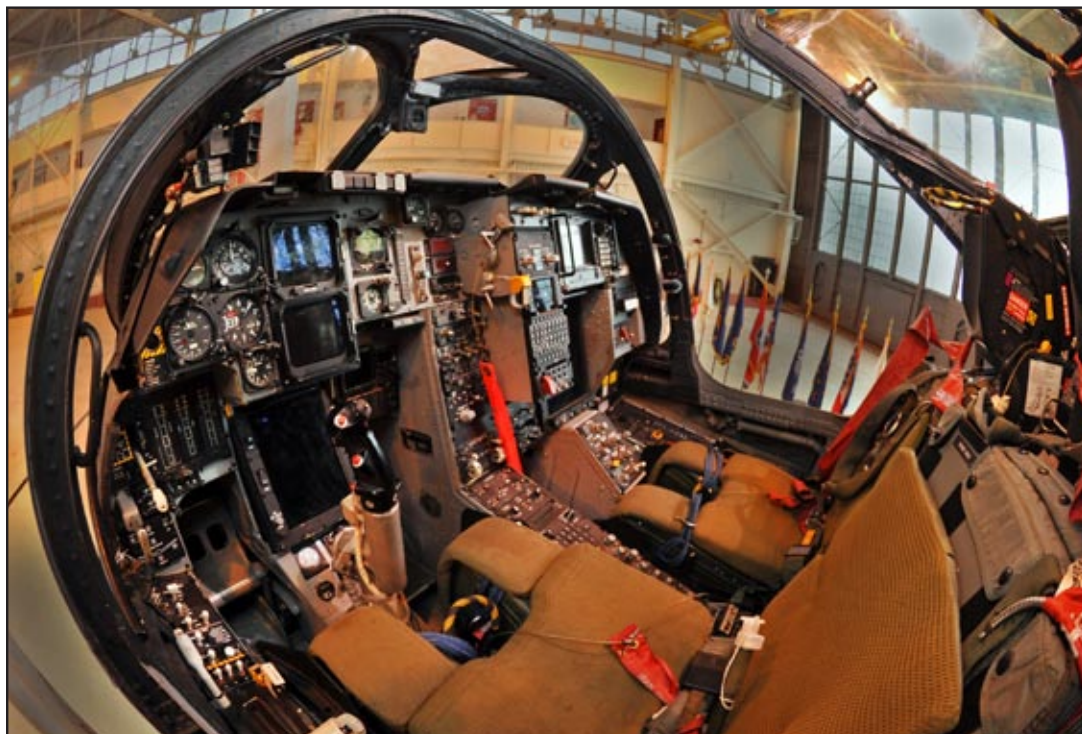
A view of the Prowler front cockpit of the ICAP III jet.
