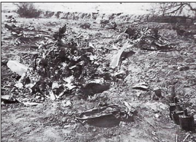
The wreckage of the Corsair . Note the backs of three .50-caliber machine guns, formerly in the right wing of the aircraft, buried on impact in the lower right-hand corner. Granados collection
